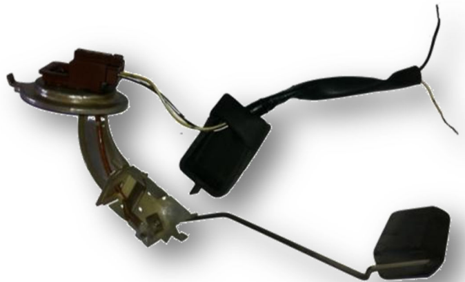
Figure 1: Fuel Sender example
